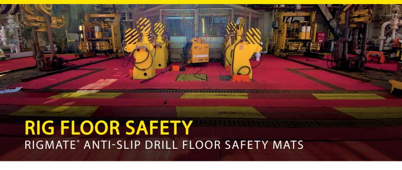
SCOTGRIP® INTERNATIONAL HD Rigmate® is a heavy duty, high traction anti-slip polyurethane rubber mat for use on drill floor rotary areas. Our unique Pyragrip® anti-slip safety surface is fully integrated with our substrate; steel pins are not necessary in our products.
