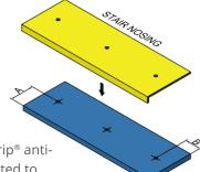
Stair tread to which Scotgrip® antislip stair nosing is to be fitted to.
